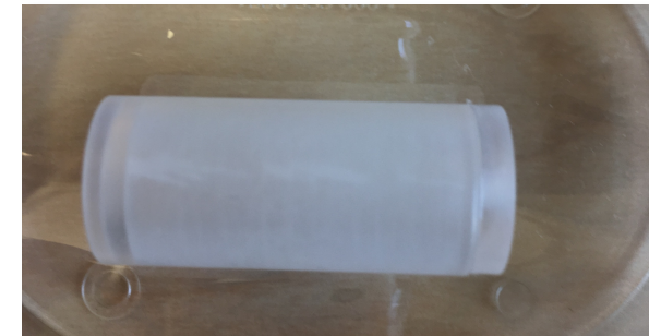
Early stilbene cell prototypes developed with Inrad Optics
