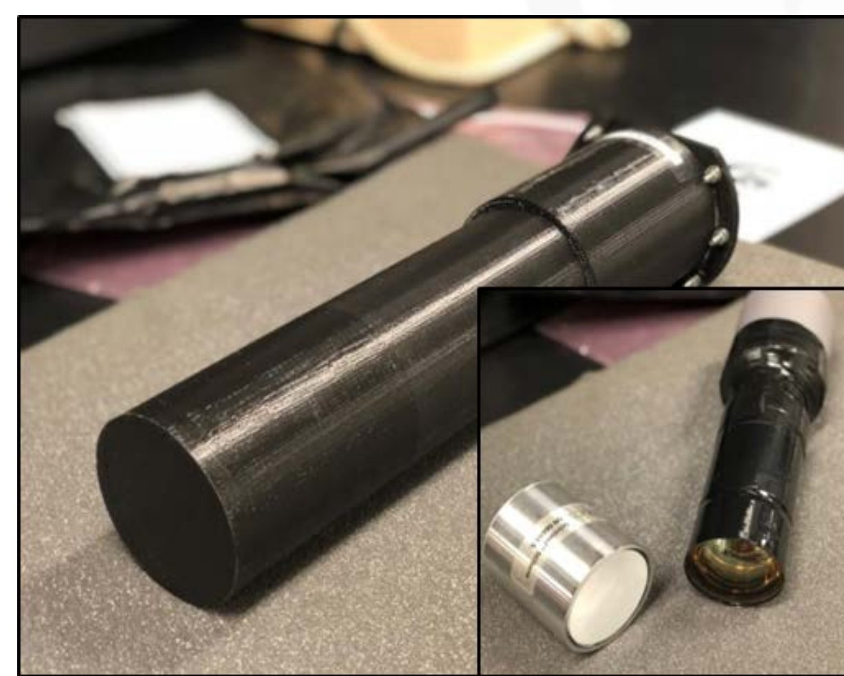
Fig. 2. Trans-stilbene crystal and ET 9214B PMT couple.
