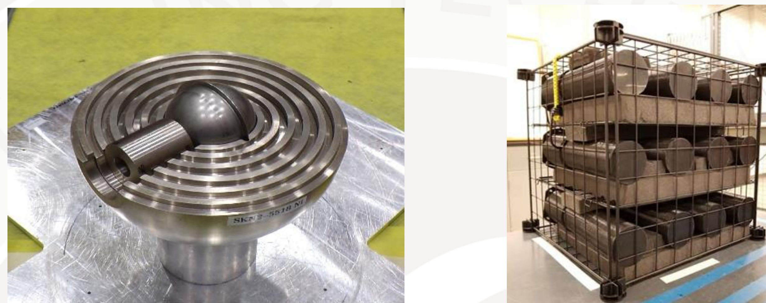
Fig 4. (Left) Ni-reflected assembly used in measurement. (Right) Photo of the measurement system.
