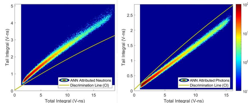
Fig. 3: ANN-attributed neutrons (Left). ANN-attributed photons (Right). The yellow line is the discrimination line used in CI PSD. The ANN successfully discriminated this PuBe data even though it was trained with <sup>252</sup>Cf only.
