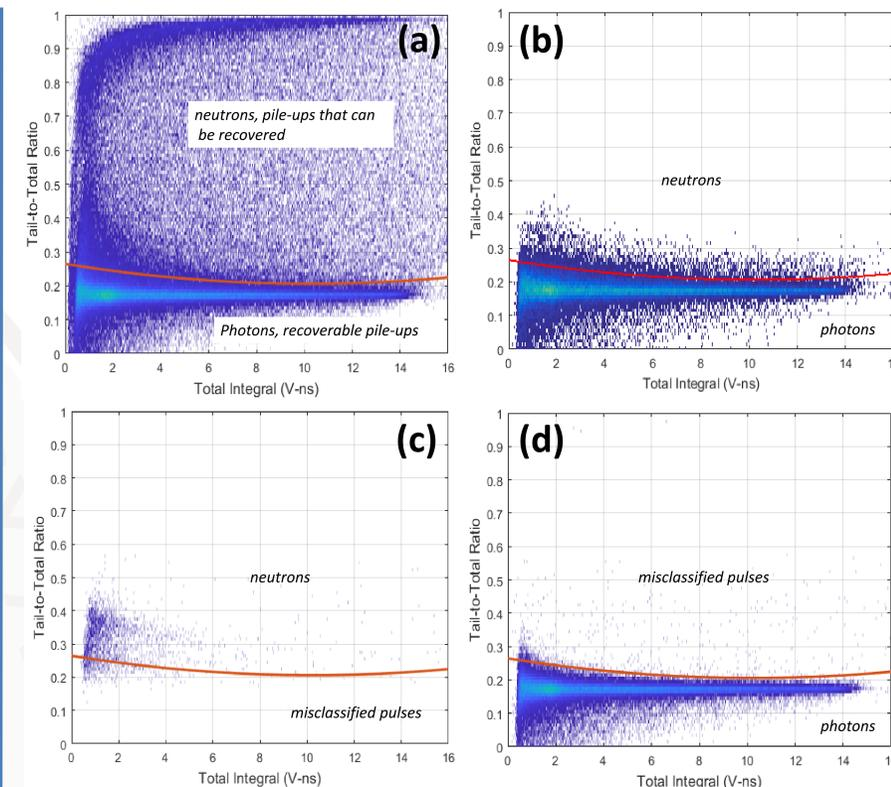
Fig. 4: Results for a 2" stilbene detectors during DU active interrogation. Comparing recoverable ANN data (a) to classifiable CI data (b) illustrates the potential advantage of ANN compared to traditional CI. ANN-attributed neutrons (c) and ANN-attributed photons (d) appear in the region predicted by CI PSD. The red lines are the discrimination line used in CI PSD.
