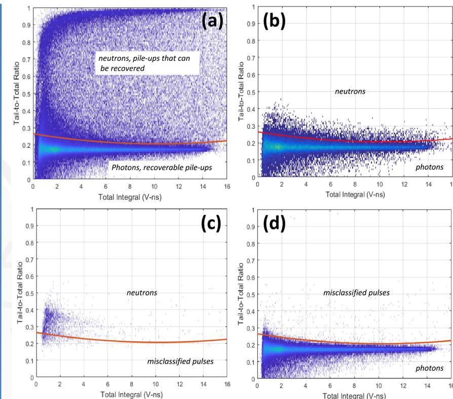
Fig. 4: Results for a 2" stilbene detectors during DU active interrogation. Comparing recoverable ANN data (a) to classifiable CI data (b) illustrates the potential advantage of ANN compared to traditional CI. ANN-attributed neutrons (c) and ANN-attributed photons (d) appear in the region predicted by CI PSD. The red lines are the discrimination line used in CI PSD.
