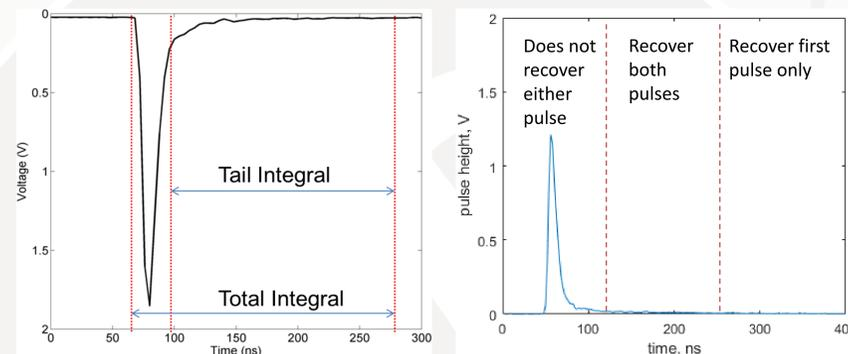
Fig. 2: Example voltage pulse from a stilbene organic scintillator, with labels for PSD (Left). The pulse recovery by the ANN is dependent on the separation time (Right).
