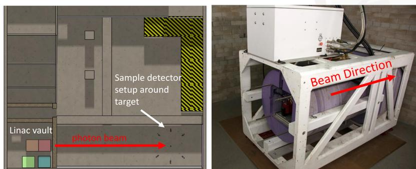
Fig. 1: Lab space, dimensions: 20 m x 15.7 m (Left) and linac in concrete vault (Right)
