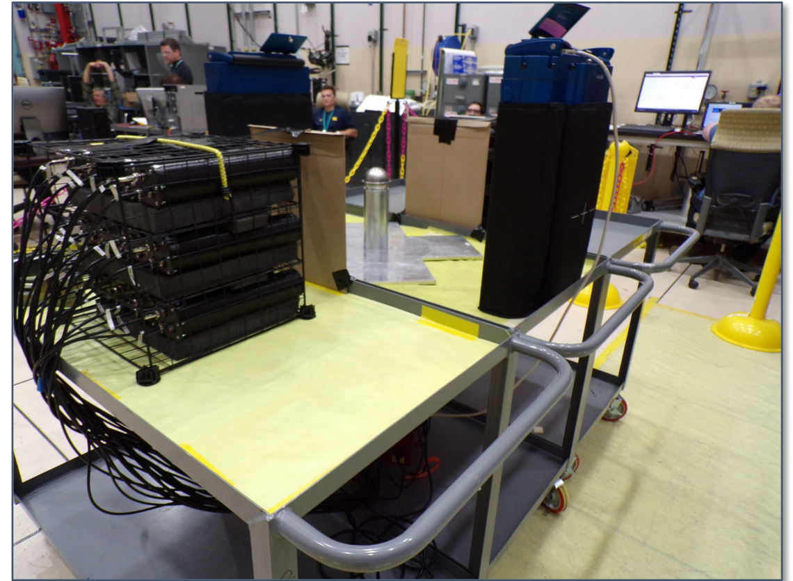
An image of the experimental setup with the BeRP ball and tin-copper graded shields
