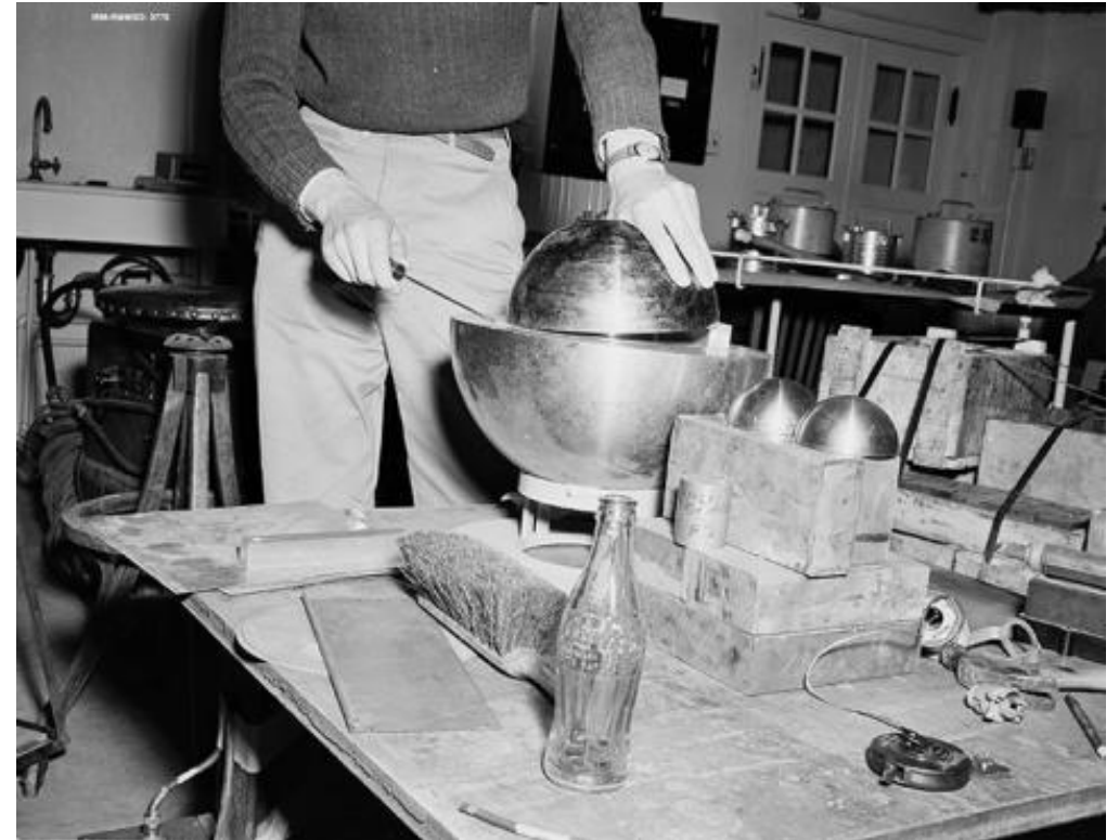
Louis Slotin separating plutonium hemispheres with a screwdriver
