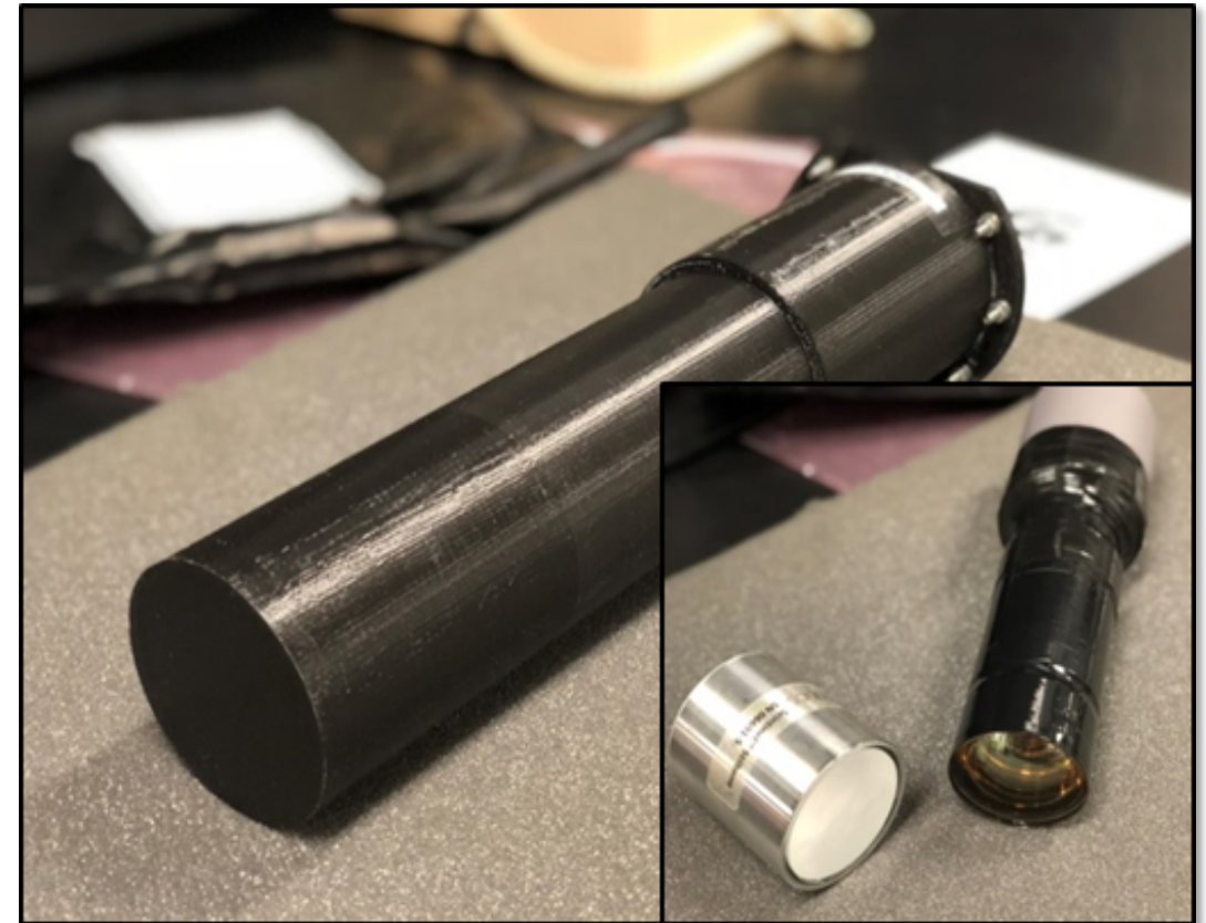
Trans-stilbene crystal and ET 9214B PMT couple.
