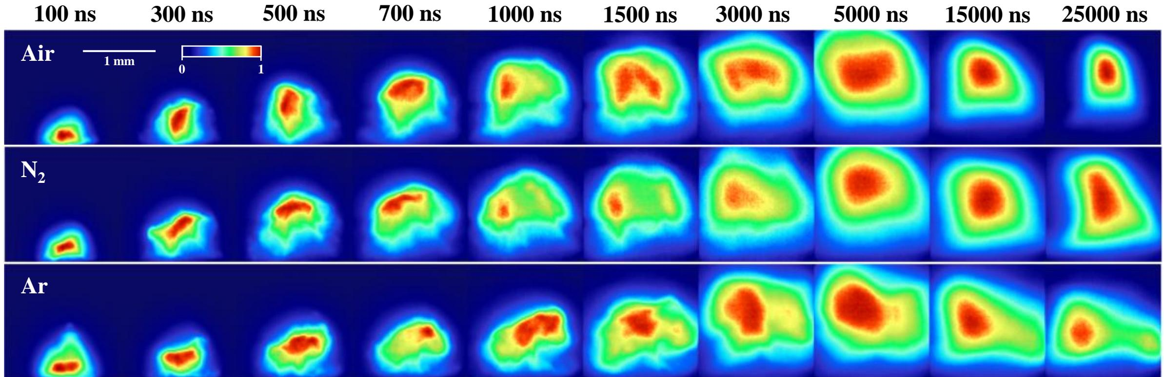
(1) Faster decay in total emission intensity in air compared to N<sub>2</sub> (2) Stronger emission in Argon due to higher gas density
