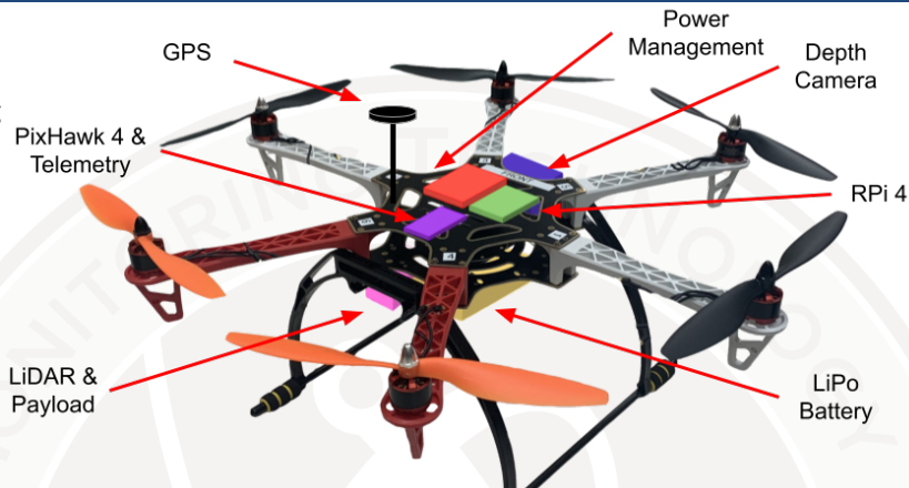
Figure 1: Modified DJI F550 drone kit showing focal points of individual undergraduate student efforts to be integrated into the system.
