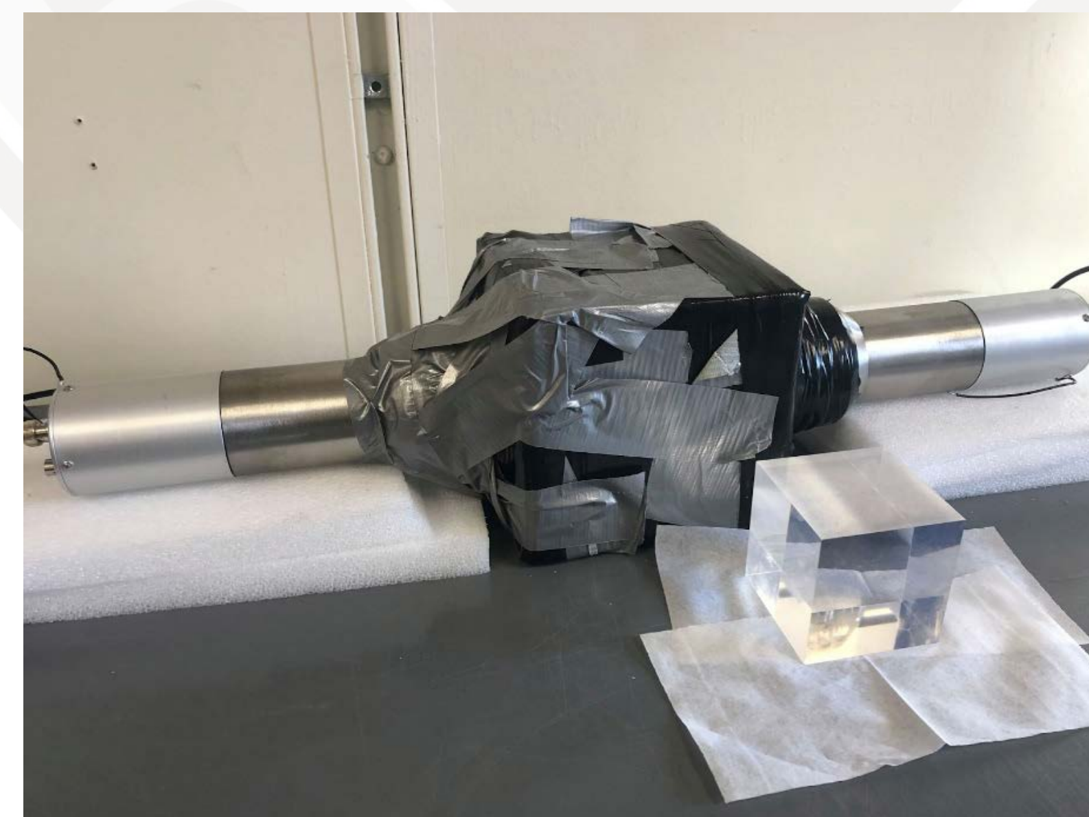
Figures 3 and 4. 6-in side length 1D scatter camera prototype and neutron scatter position calibration curve
