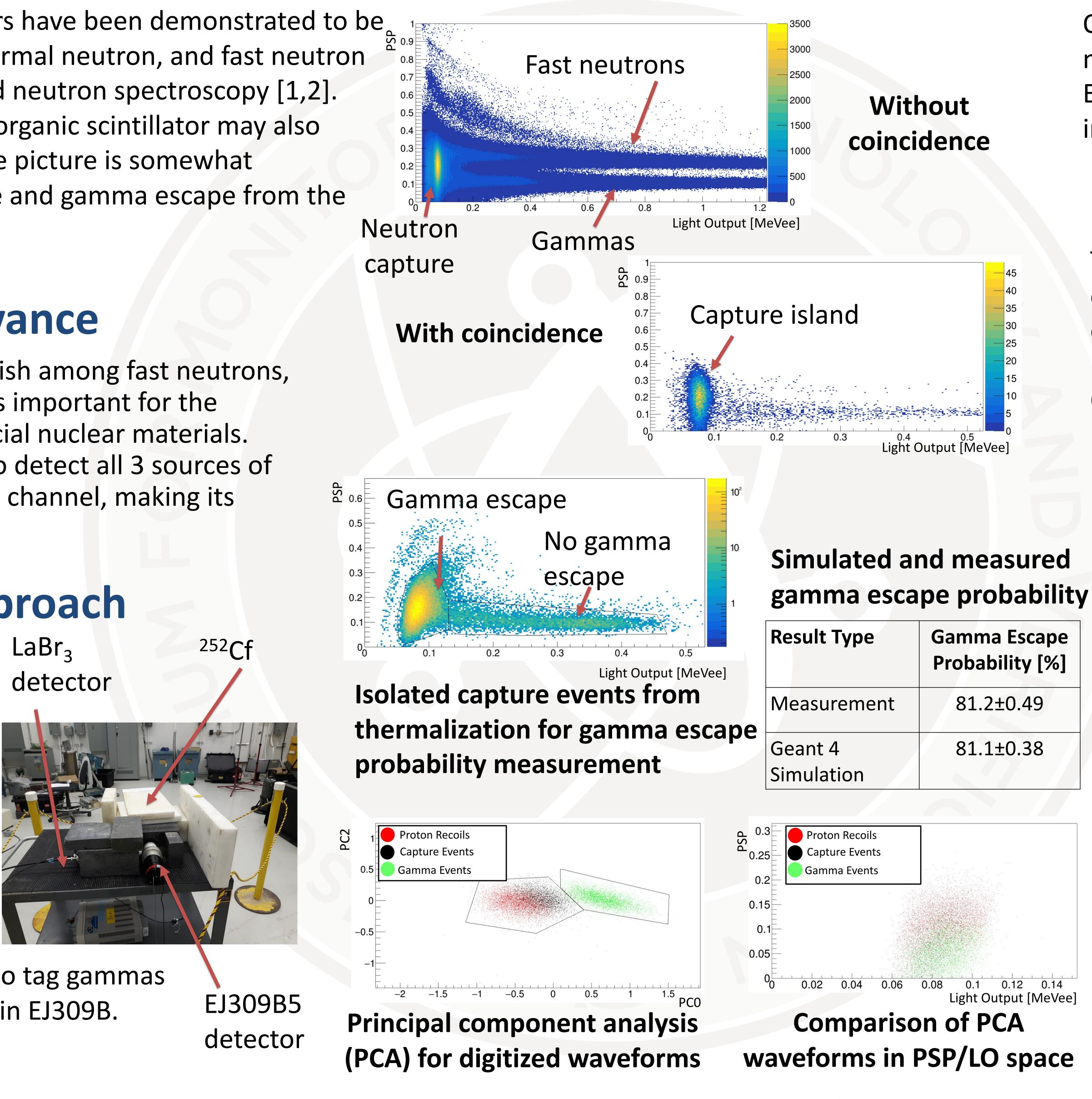
We use a LaBr<sub>3</sub> detector to tag gammas from <sup>10</sup>B neutron capture in EJ309B.
