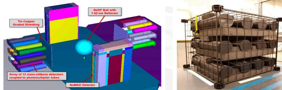
Fig. 3. (Left) Model of experimental setup and detection system measuring the BeRP ball and (Right) 3x4 array of trans-stilbene detectors
