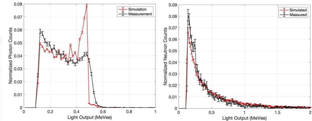
Fig. 4: <sup>137</sup>Cs normalized photon spectra (Left). <sup>252</sup>Cf normalized neutron spectra (Right).
