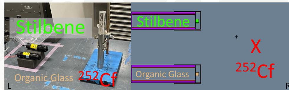
Fig. 3: <sup>252</sup>Cf measurement setup (Left). MCNP cutaway of measurement simulation model (Right). Organic glass detector results not analyzed in this work.
