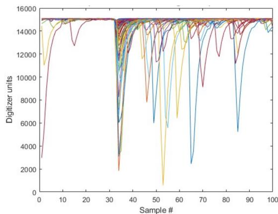
Fig. 1: Example pile-up pulses in stilbene during DU interrogation. These pulses are rejected as they would be falsely attributed as neutrons
