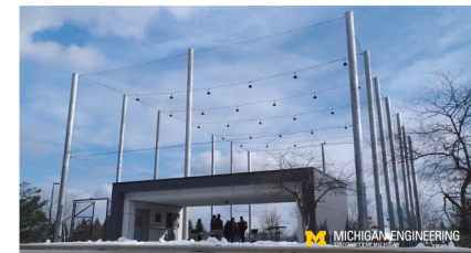
A purpose-built 930 m 2 netted scientific facility, M-AIR, was used to successively test at progressively higher lifts and longer motions at greater speeds.
