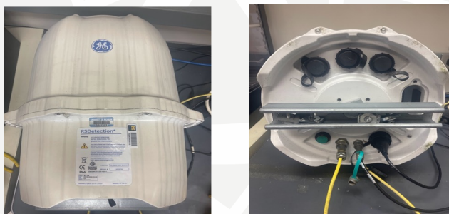
High Pressure Ion Chamber and interface panel ▲
