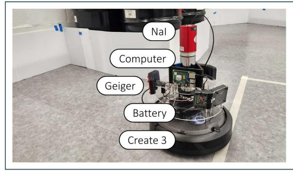
Nal detector binning provides 2.54-times faster coverage
