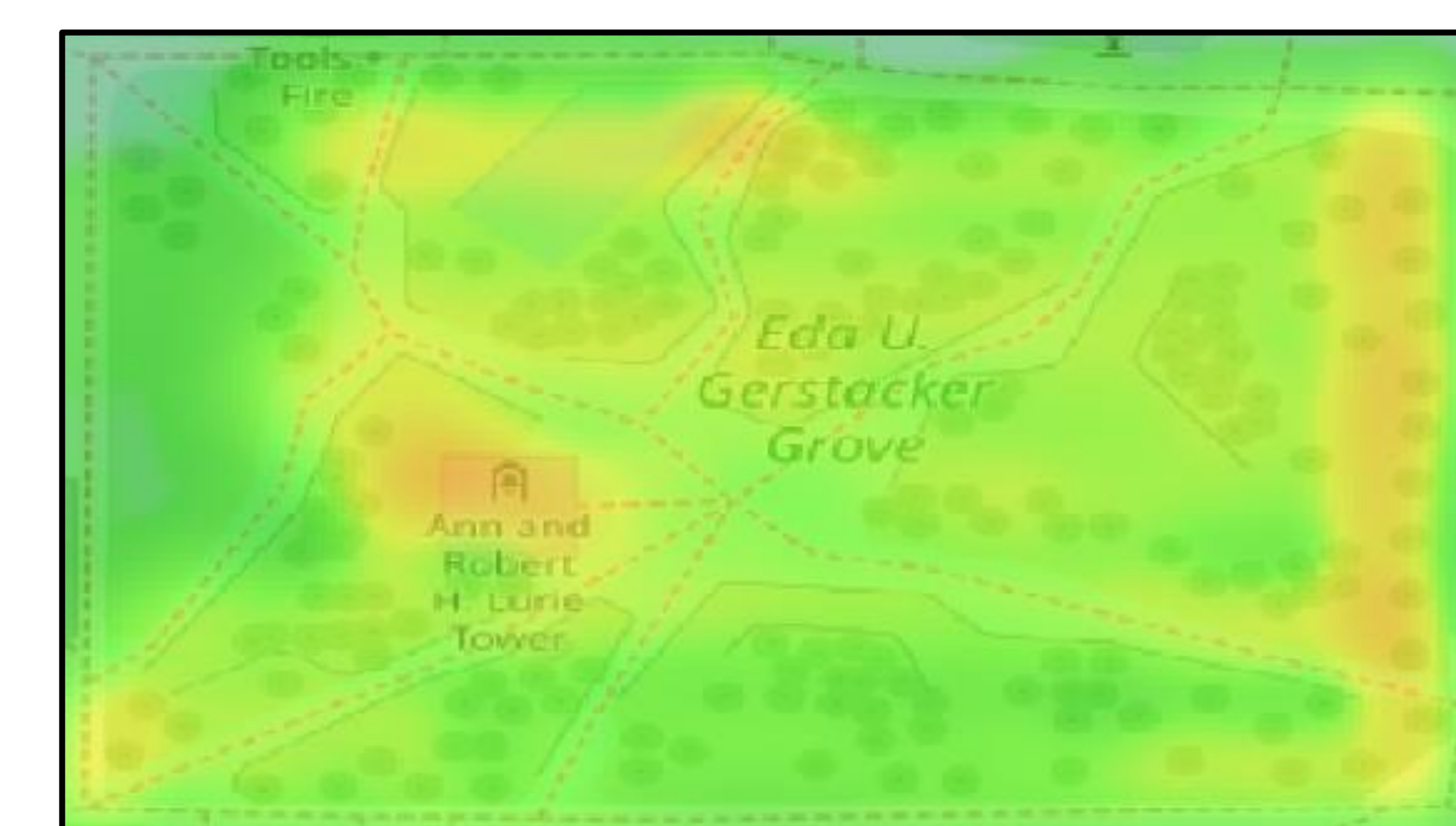
Map of radiation field in Eda U. Gerstacker Grove using Ludlum model 12s survey meters with Counts-Pro mapping software.
