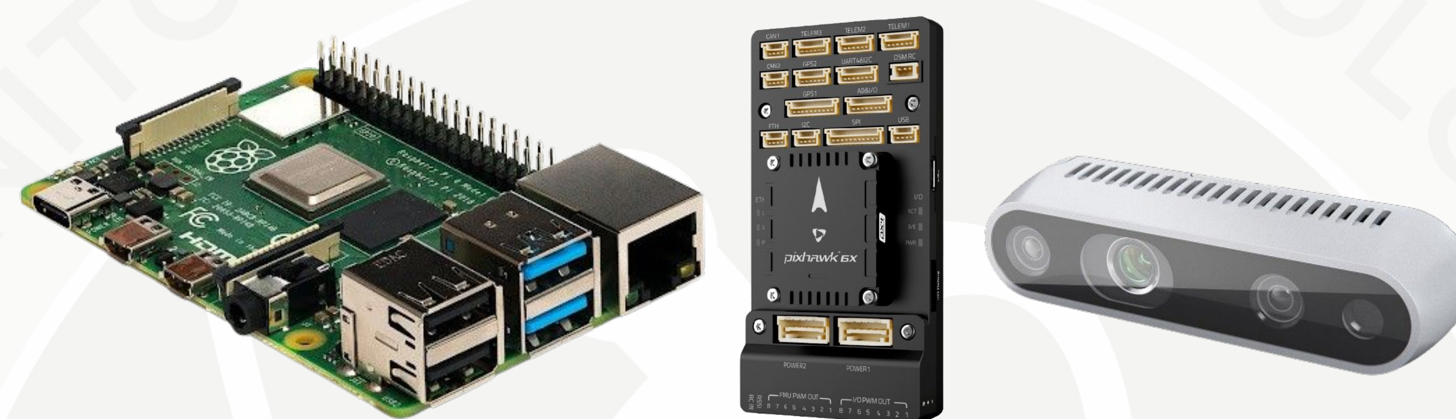
Figure 2: Raspberry Pi, Pixhawk Flight Controller, Intel Depth Camera
