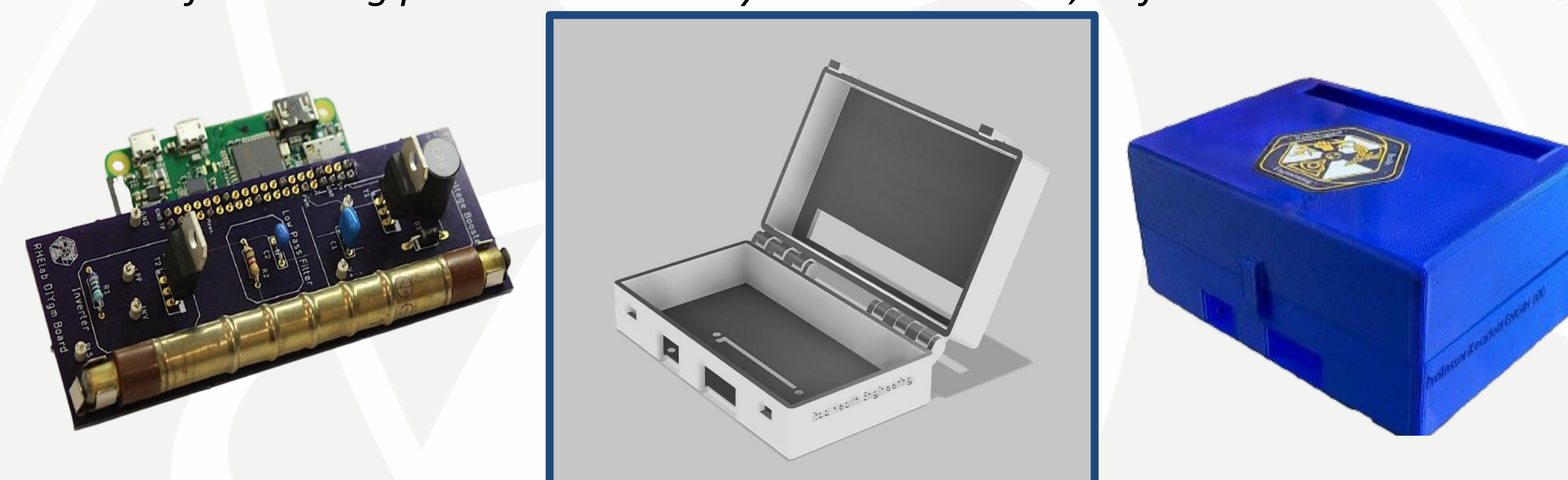
Design of Do-It-Yourself Geiger-Mueller Counter (DIYgm) and case.
