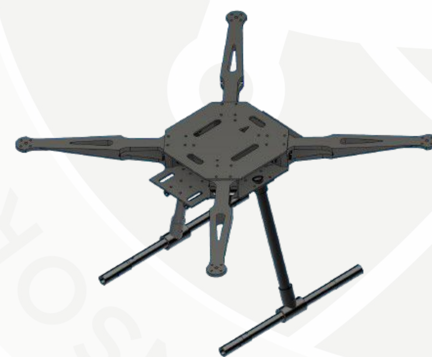
▲ Drone Frame CAD Assembly
