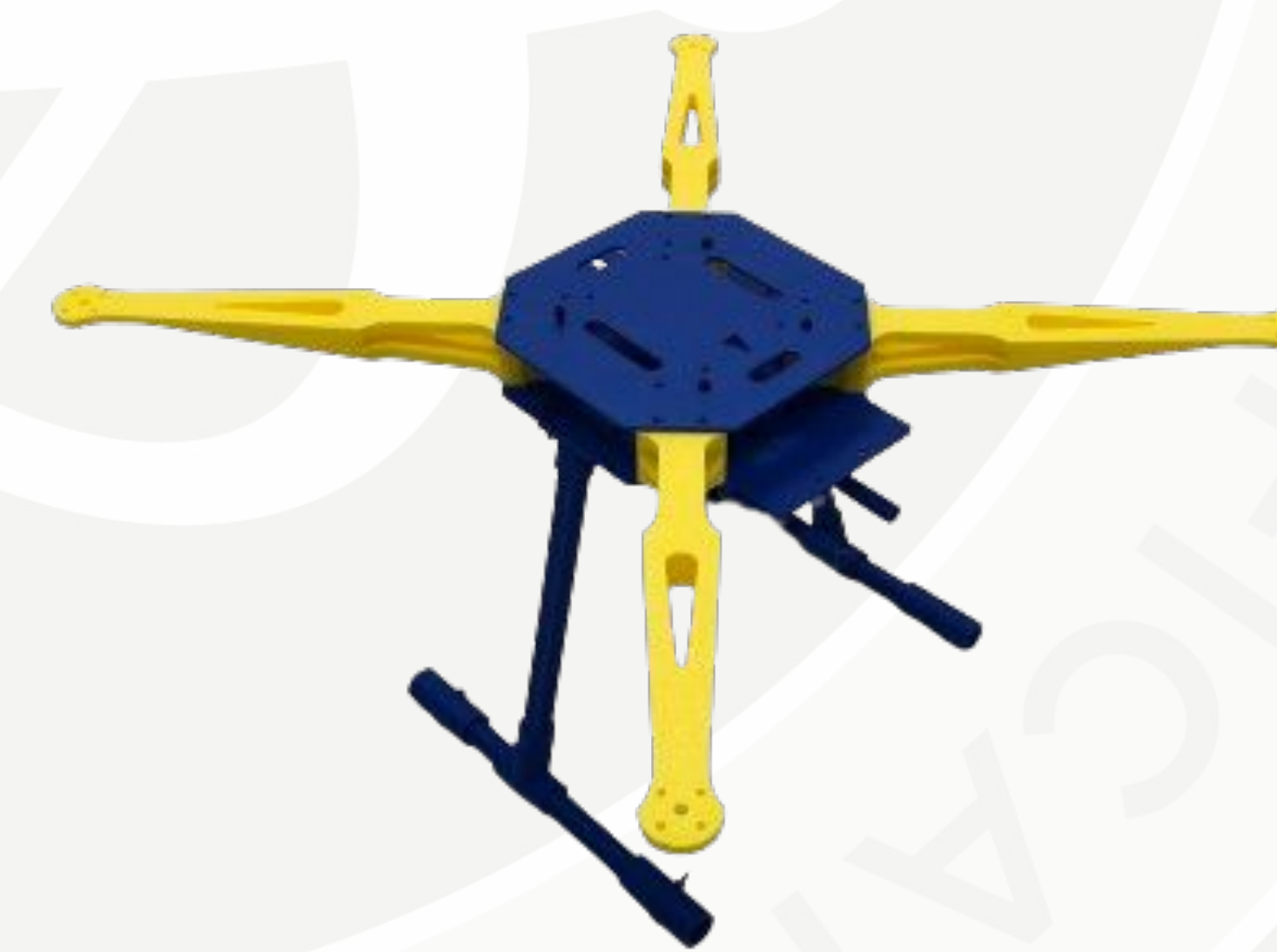
▲ 3D Printed Drone Frame
